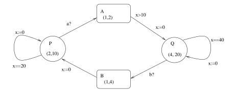
Figure 5. Timed Automaton with Periodic and Sporadic Tasks.
